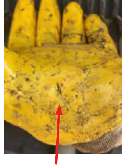
Hole in glove made by high pressure jet
