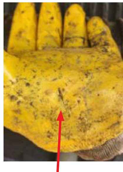
Hole in glove made by high pressure jet
