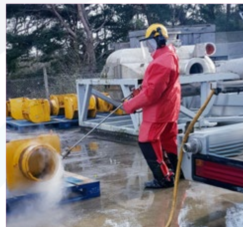
An operative carrying out high pressure water jetting using a lance that is compliant with the WJA Code of Practice and wearing specialist PPE
